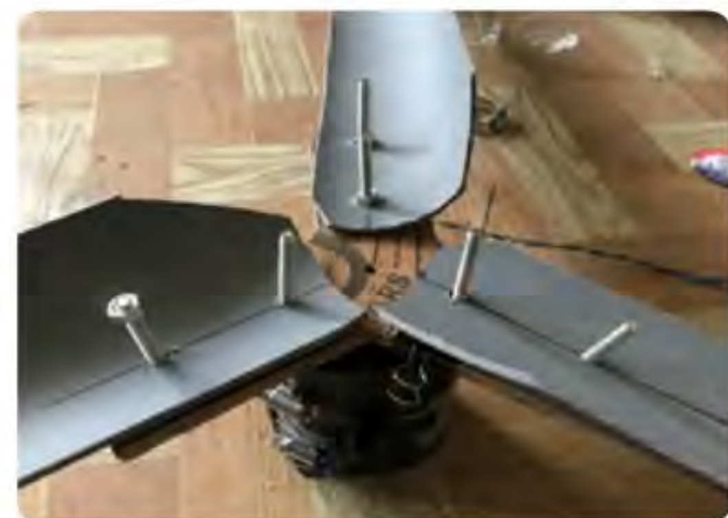
Figure 10: Blade attachment to generator
