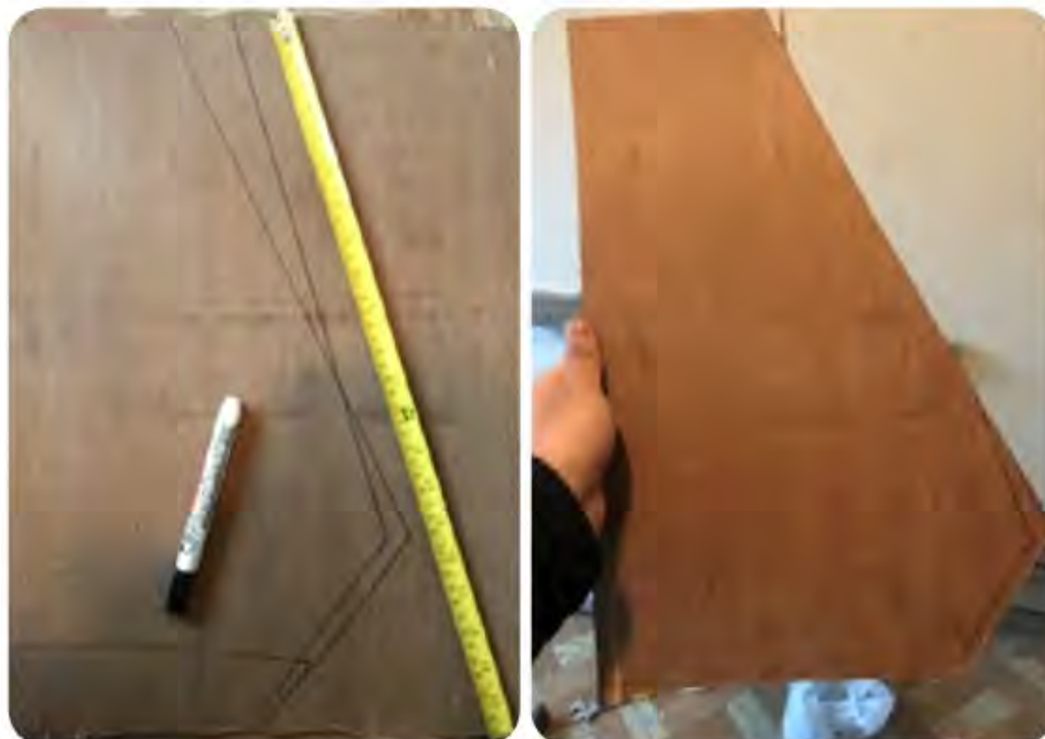
Figure 8: Tail fin cut out
