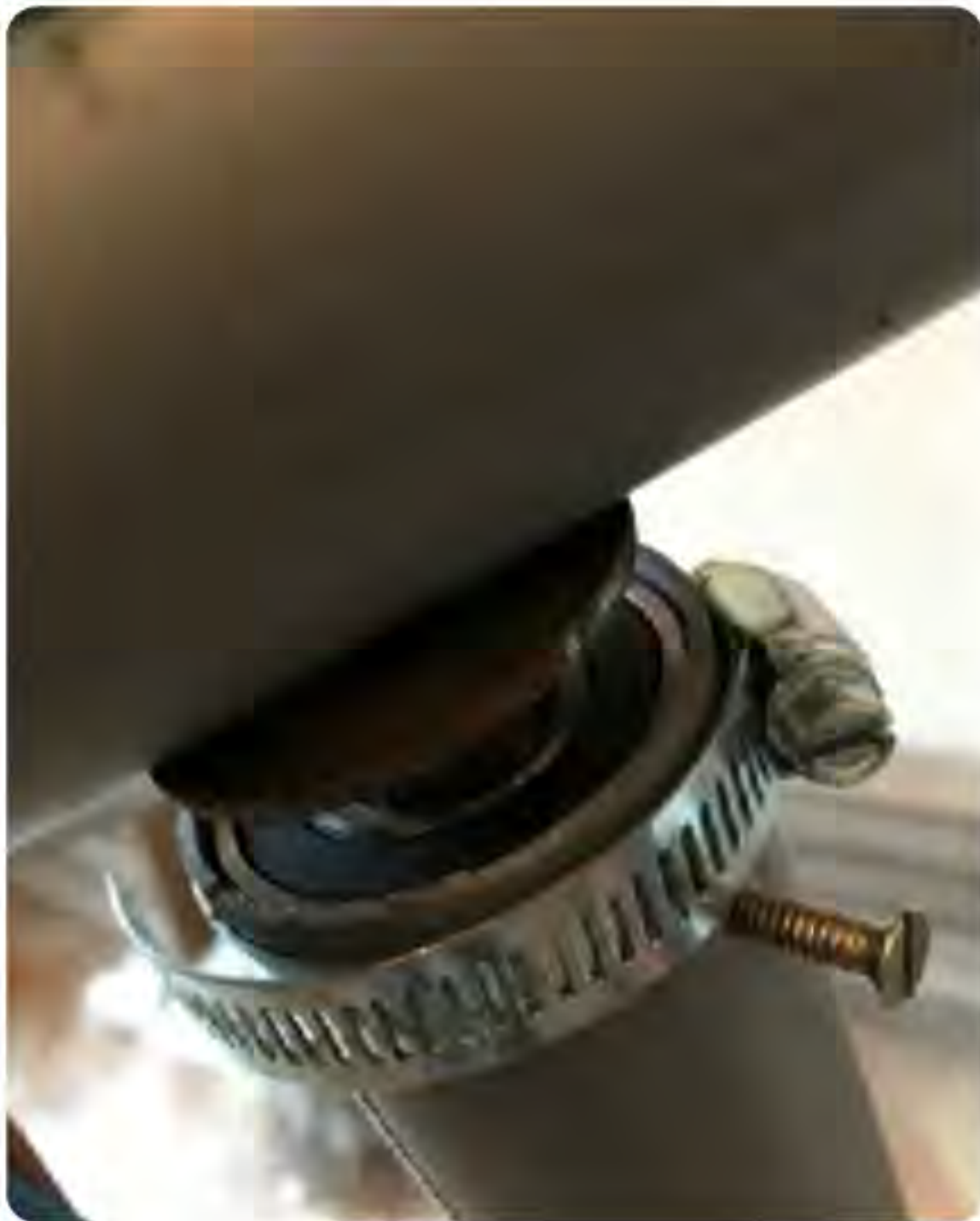
Figure 11: Yaw Axis attachment for rotation
