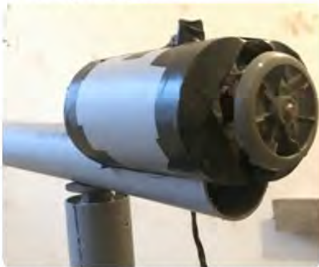
Figure 7: Generator Fastening
