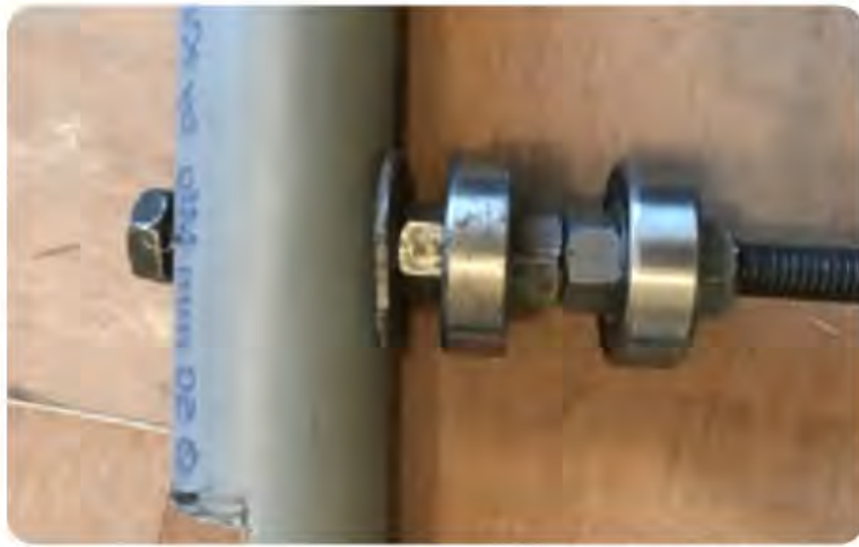
Figure 6: Attaching Yaw shaft to tail boom
